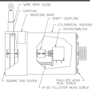
HX Series Transducer Cutaway View
