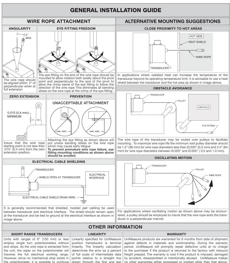
the potentiometer, it is possible to continue extracting the wire rope beyond the working range of the transducer. When this occurs, the wiper of the potentiometer passes through a dead zone where no electrical output is observed and then begins at the zero output position again and repeats its output. Although the full extension of the wire rope may, in some cases, approach 12" (300 mm) the working range occurs from initial extension.
