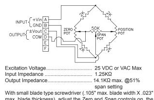
max. blade thickness), adjust the Zero and Span controls on the transducer to set zero voltage output and maximum output voltage as follows.
