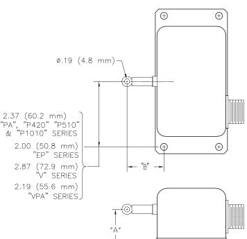
$^{*}$  With "DS" (dust shield) option, add 0.36" (9.1 mm) to "B" dimensions above.
