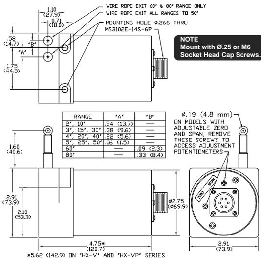
Note: Dimensions in brackets are millimeters.
