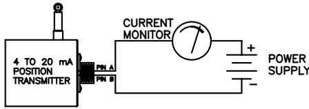
The 4 to 20 mA output transducer is a 2-wire, loop powered device. The transducer, power supply, and current monitor must be connected in series as illustrated above.
